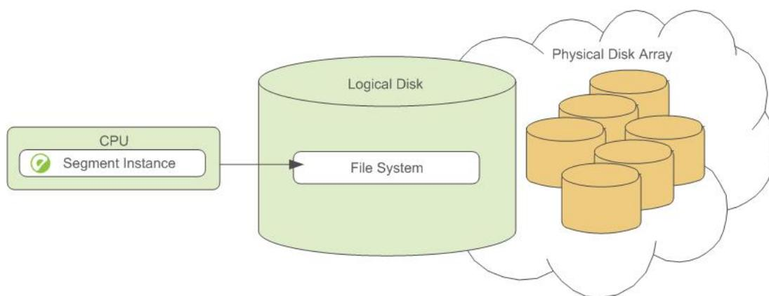
**Figure 4: Logical Disk Layout in Greenplum Database**
