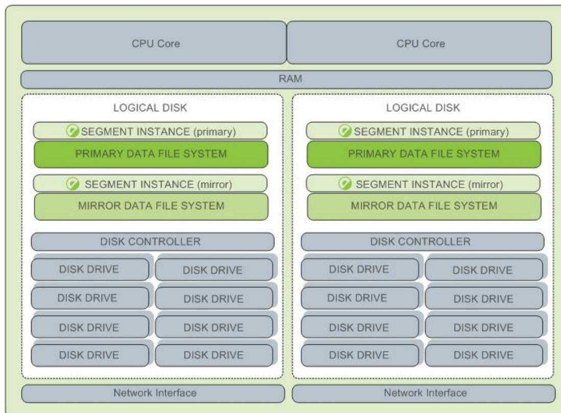
**Figure 3: Example Greenplum Database Segment Host Configuration**
